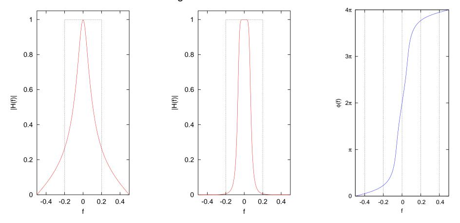
Left: Transfer function of Butterworth filter of order 1. Middle: Transfer function of Butterworth filter of order 4. Right: Phase of Butterworth filter of order 4.
