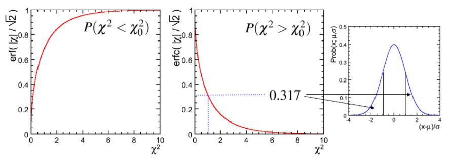
★ This is nothing more than a different way of expressing a 1D Gaussian distribution (or more correctly its two-sided integral)
