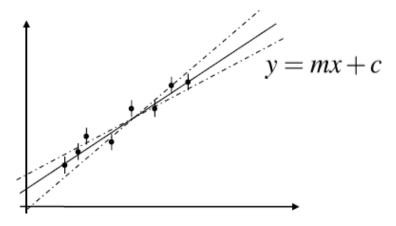
★ Suppose we want to calculate the error on y as a function of x based on our fit:
