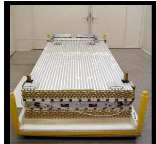
A module with 2x4 layers of drift tubes (ATLAS)
