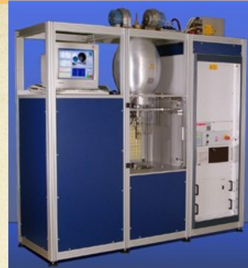
Plasma reactor for growing diamond.
